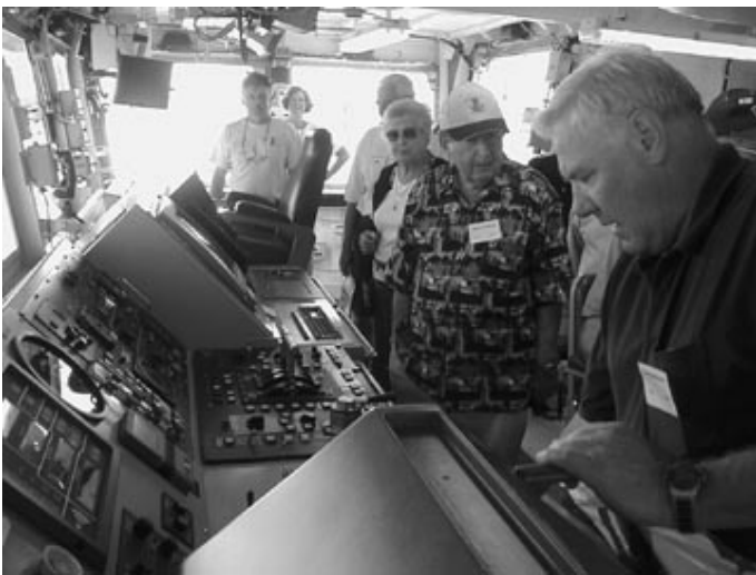
The computer-controlled 175 foot buoy tender James Rankin (WLM 555) has no wheel. It is controlled by computers and a lever. It has a bow thruster and 360 degree Z-drive propulsion so that it can move sideways.
